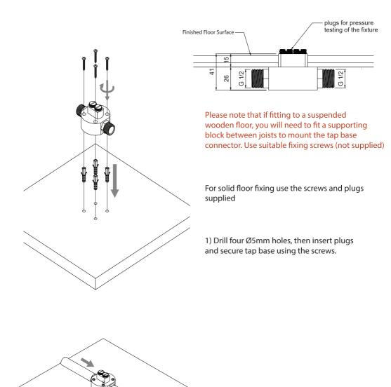
2) Connect the hot and cold water supplies to
