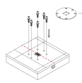
3) Using the securing plate as a template, mark the six holes and drill using an 8mm bit and insert the six plastic plugs provided.
