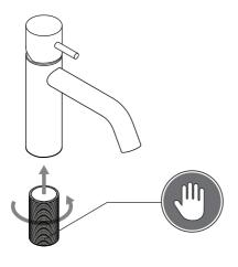
1) Screw the threaded brass connector into the tap body and hand tighten
