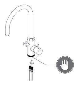
4) Screw the flexible hoses into the inlets on the tap body and hand tighten.
