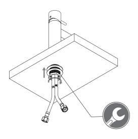
4) From beneath, fit the rubber washer followed by the metal washer and secure using the locking nut. Finally connect the flexible connections to the hot & cold supply.
