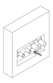
1) Install the built in part into the wall and secure. Connect the hot & Cold supply pipework, to the corresponding inlets of the tap body. Carefully check the depth before finishing / tiling the wall.
