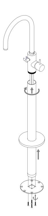
5) Insert the flexible hoses into the column, and then screw the column to the mixer body.
