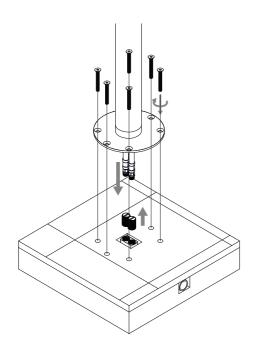
8) Screw the flexible connectors into the tap base. Then fix the column to the floor using the screws supplied.
