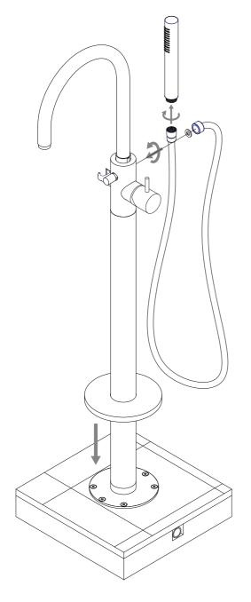
9) Fit the shower hose to the mixer outlet. Ensure the washer is fitted. Then connect the Hand-shower to the hose.
