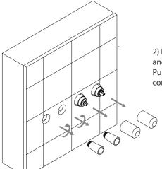
2) Remove the plastic plugs from the spout outlet, and the handset wall outlet by un-screwing Pull off the two plastic caps from the flow and diverter controls
