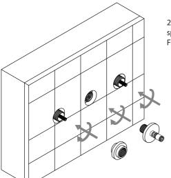
2) Wrap some PTFE tape onto the thread of the spout connector, and screw into the tap body. Fit the wall plates by screwing onto the tap body.
