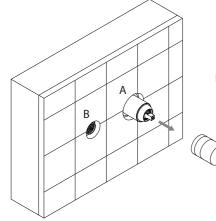
3) Carefully fit the wall plate, using a small bead of silicon sealent, to fix into position.
