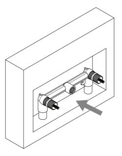
1) Install the built in part into the wall and secure. Connect the hot & cold supply pipework to the corresponding inlets of the tap body. Carefully check the depth before finishing / tiling the wall. Allow access holes of no more than 40mm for each control in order to service the flow cartridges.
