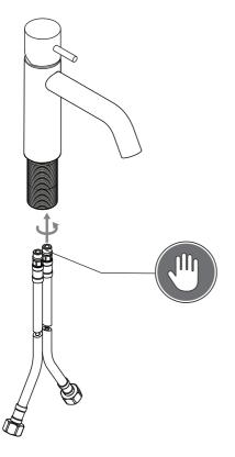
2) Screw the flexible hoses into the water inlets of the tap body and hand tighten
