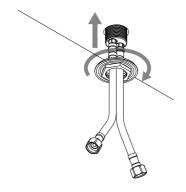
5) Holding the spout, fit the rubber washer, then the metal washer, and secure by fitting the locking nut and tightning.
