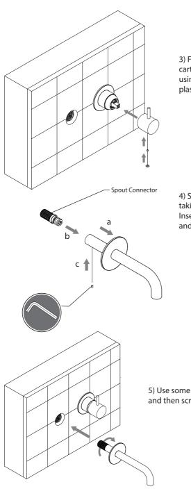
3) Fit the control handle on to the flow control cartridge, and secure by tightning the grub screw using a 2.5mm allen key. Finish by inserting the plastic cap into the grub screw hole.
