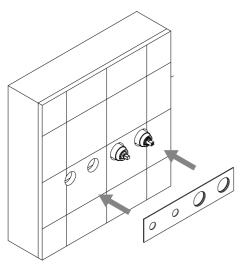
3) Fit the concealing plate and secure using a small bead of silicon sealent.
