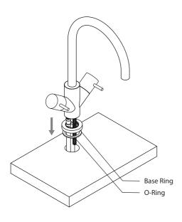
3) Fit the base ring and o-ring on to the tap body, and then insert the tap into the tap hole.
