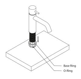
3) Fit the base ring and o-ring on to the tap body, and insert the body in to the tap hole.
