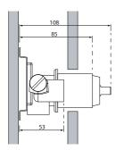
1) Fit the concealed part into the wall cavity, using the fixing holes (F) Pay careful attention to the depth. Check the concealing plate dimensions before making any holes in the finished surface. Connect the hot & cold water supply to the inlets.
