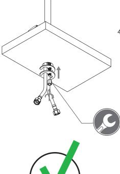
4) From beneath, fit the rubber washer. followed by the metal washer. Then fit the locking nut on to the threaded rod and tighten using a spanner. Finally connect the flexible connectors to the hot and cold supply.
