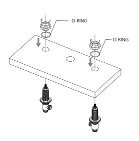
1) Firstly fit the locking nut, metal washer & rubber washer to each deck valve. Insert each deck valve trough the tap hole from underneath. From the top, fit the o ring to the deck flange and screw down onto the valve until it locks then, secure each valve by tightning the locking nut.
