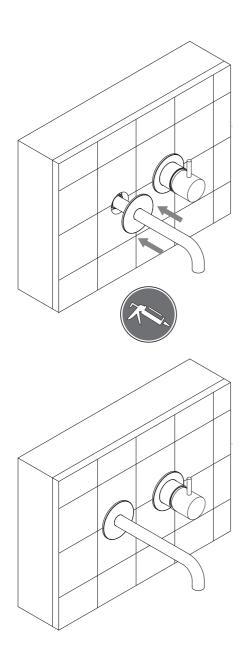
6) Carefully slide the spout wall plate back to the wall and secure using a small bead of silicon sealent.
