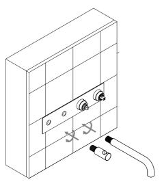
4) Wrap some PTFE tape around the thread of both the spout thread and the hand shower support thread. Screw the spout into the tap body. Screw the hand shower support in to the tap body.
