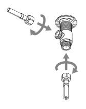
6) Fit the flexible connectors from the spout to the outlets on each deck valve. Connect Hot and Cold water supplies to each deck valve.
